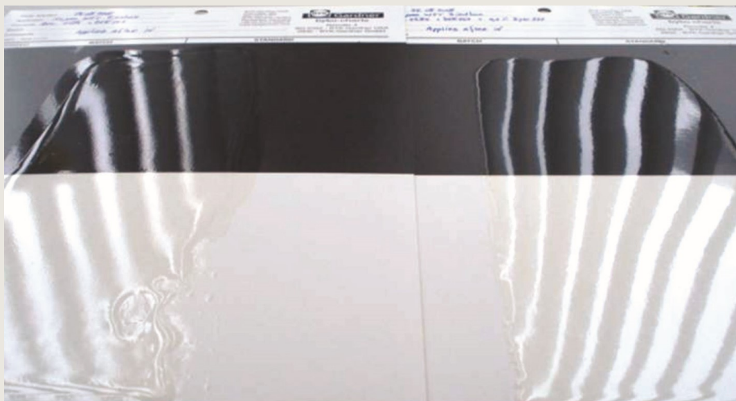
FIGURE 6: APPEARANCE OF 75 μ CLEAR COATS APPLIED WITHOUT ADDITIVES (LEFT) AND USING A LEVELING ADDITIVE (RIGHT), FOLLOWING A 10 MINUTES INDUCTION TIME. ANCAMINE 2685 CURING AGENT WAS MIXED AT 48 PHR WITH A BIS-A/F EPOXY RESIN DILUTED WITH EPODIL® 748, EEW195, μ.900 MPA.S
