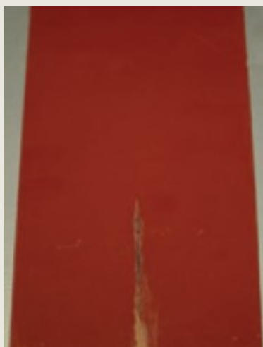
FIGURE 4: ANCAMIDE® 2864 PRIMER AFTER 2000 H OF SALT SPRAY PERFORMANCE
